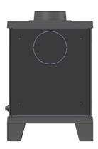
Remove the panel from the stove by unscrewing the four screws and then remove the circular cut out for rear flue installations. Replace the rear heat shield.
