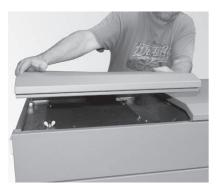
Fig. 133 Removing the rear cover
