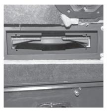
Fig. 18 Sliding the ash removal device into the designated guides
