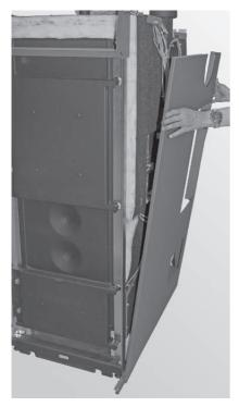
Fig. 51 Hooking on the side panel
