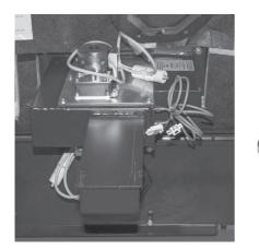
Fig. 20 Screwing on the ash removal device
