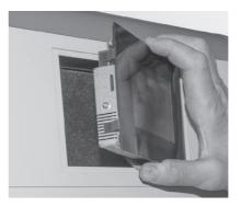
Fig. 89 Inserting InfoWIN Touch into the operating panel
