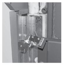
Fig. 38 Routing the door safety switch (only at PuroWIN PWPE 60)
