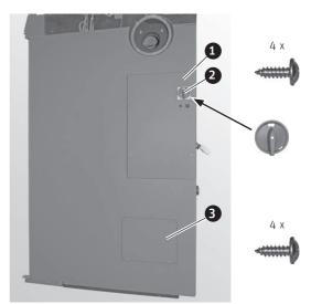
Fig. 54 Installing the knob of the main switch, the cover for control panel 1 and the cleaning cover
