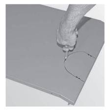
Fig. 97 Punching out the cut-out on the rear cover if the flue connection is at the top
