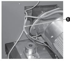
Fig. 148 Tying the cables together using cable ties
