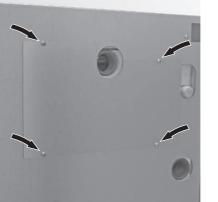
Fig. 67 Installing the cover for the cleaning linkage
