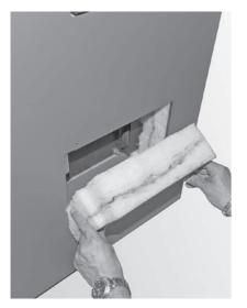
Fig. 53 Inserting the insulation into the cleaning opening
