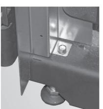
Fig. 31 1 screw at front of base
