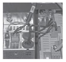
Fig. 144 Connect the mains filter and frequency converter, cables and earth; connect the plugs
