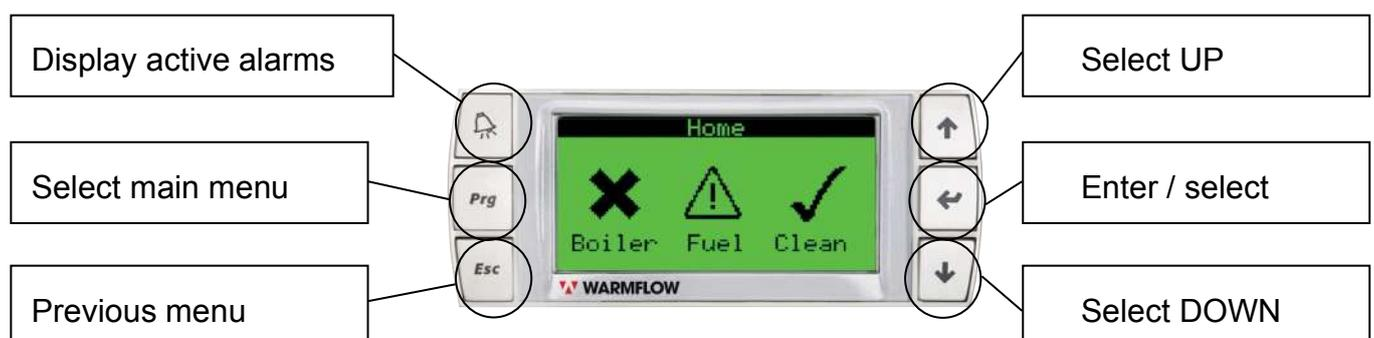
**Figure 3: User Control Interface and Function Keys.**
