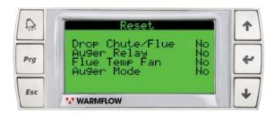
Figure 90: Engineer Reset Screen
