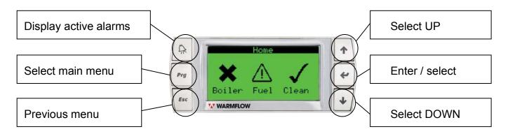
Figure 3: User Control Interface and Function Keys.
